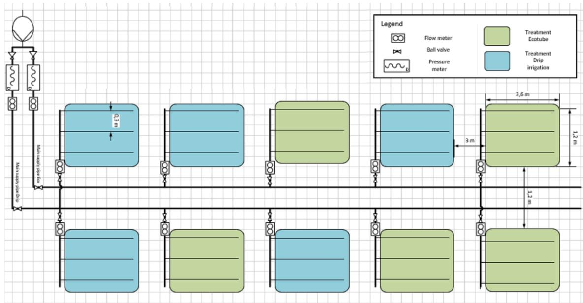
**Figure 2.** Sketch of the experimental set-up to compare drip irrigation and porous pipe irrigation
