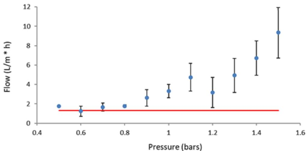
**Figure 3.** Water discharge of ecotube porous pipe at different levels of pressure. Points represent the average of five flow measurements and error bars the mean standard deviation. 1.3 L/m\*h is the nominal discharge rate at the recommended operation pressure of 0.6 bars
